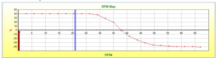
In the above example the Map signal on the top graph will cancel the any cam movement on light load regardless of the RPM of the engine. Then on high load it will activate the cams. But on high RPM the cam movement will be deactivated regardless of the load on the engine. With other words the cams will be activated only on high loads above 50% on the Map Sensor and also below 3500 RPM's.
