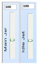
These two settings adjust the cams to a percentage of the control signal. The signal calculated above is multiplied by this % value represented by the Main and Idle Jet. The Main jet is for VVT cam on Cylinder 1 and the Idle jet is for VVT cam on Cylinder 2. This is used to balance the cams should the solenoids react differently in degrees for a certain pulse width. Always keep one at 100%.
